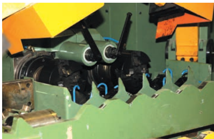
(7a) Deburring the ends
