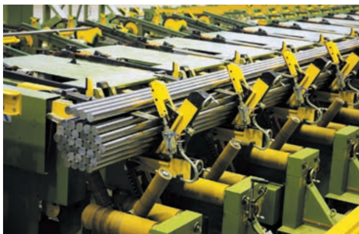
(10a) Bundling the bars together
