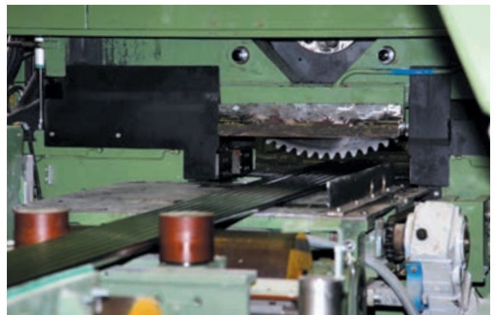
(6) Cutting bars to commercial lengths
