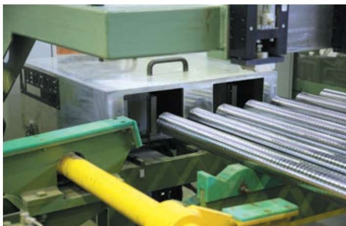
(7b) Marking the ends
