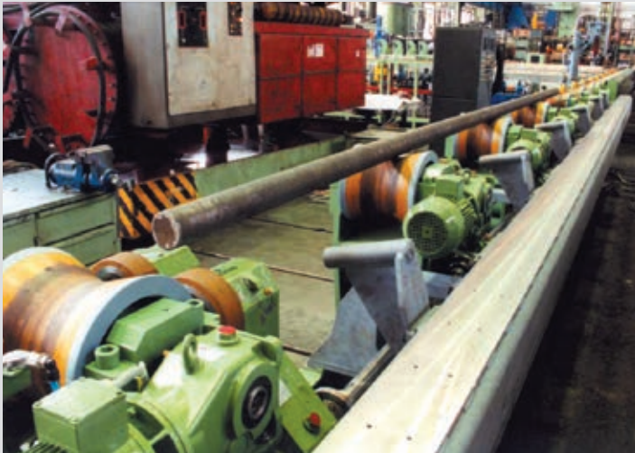
The longitudinal conveyor and round stock bundling on these lines were delivered to Sandvik, SE.
