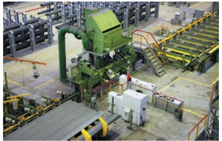
(2) Steel shot blasting of the bars
